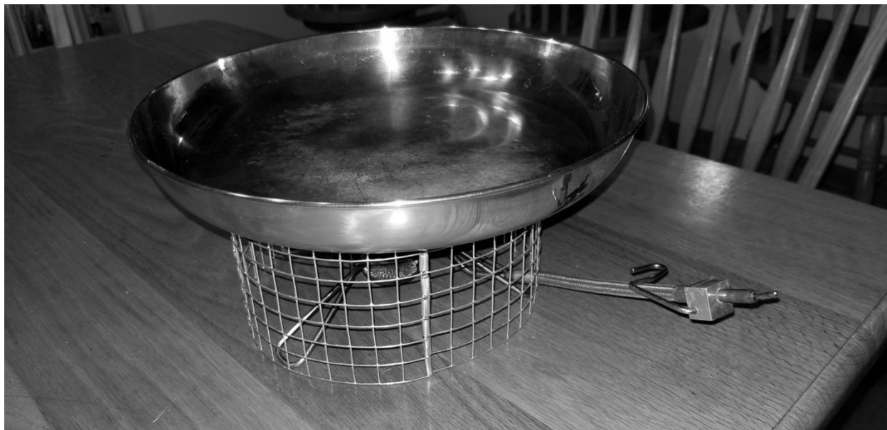
Fig. 1: Whisperlite stove and 1/2" x 1/2" hardware cloth pot support shown without windscreen
